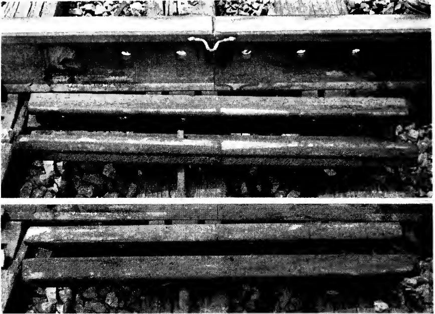
Fig. 14. South Portion Section 9, Petrolatum (Dark) (Brush coat on rail only and Plastic H receiving end plugs)
